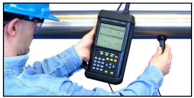
Figure 9-4: PT878GC Thickness Gauge in Operation
